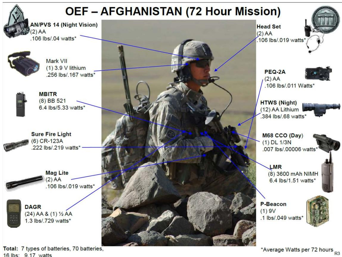
Figure 7. Operation Enduring Freedom Battery Weights
