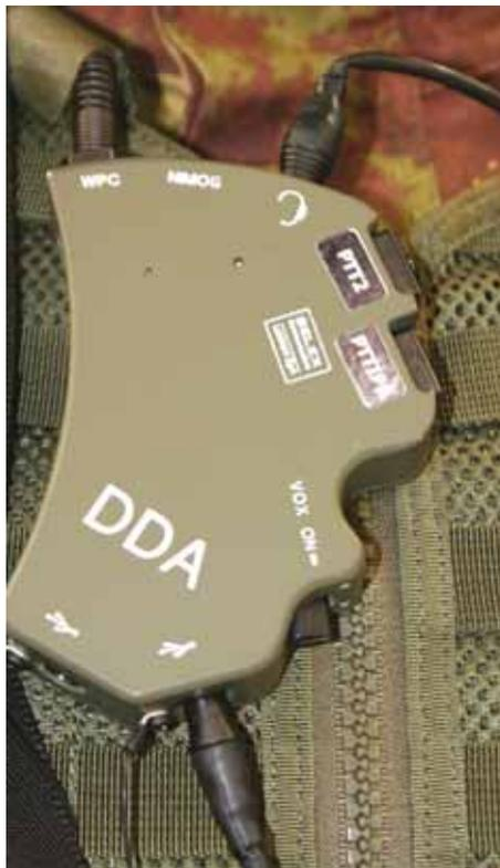
*Like other soldier modernisation programmes, Italy's Soldato Futuro uses a single control device to control worn communications and other equipment © AJB*
