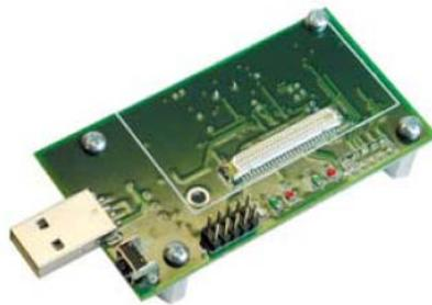
Figure 10. MIB520 Interface Board
