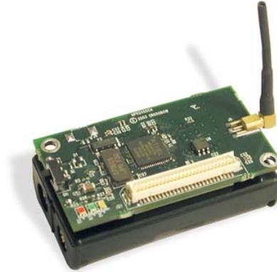
Figure 9. MICAz 2.4 GHz Mote
